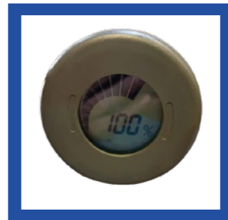
Electrical Level Meter
