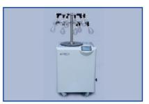
2, Ampoule tube freeze-drying rack
