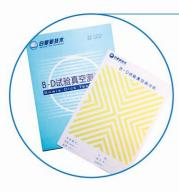
B-D vacuum-testing paper is composed of paper with air permeability and heat-sensitive dye and is used for testing remaining cold air in the process of sterilization. The color will change from light yellow to dark brown or block if no air left in chamber, and the temperature reach 132-134°C, lasting 3.5-4 min. If the conditions fail to reach certain value or there is air leakage, the color will remain light yellow or change unevenly.
